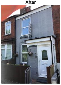
**Background:** A complaint was made under the scheme that the property was unsightly from the exterior and in a poor state of repair. A formal notice was served on the landlord under the Building Act to address the issues with the guttering and fascia's, and these were replaced in compliance with the notice, in addition to further works being carried out to improve the external appearance.
