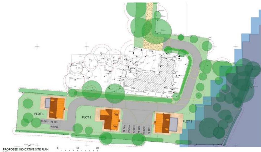
Figure 3 - Site plan overlain with flood zones
