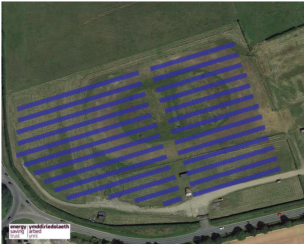
Figure 11-4 Potential layout of adjacent solar PV generation
