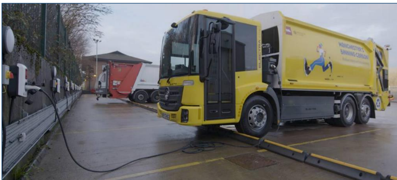
Figure 9-1: One of the City of Manchester's 27 Electra/Mercedes 26 tonne 300 kWh electric refuse vehicles
