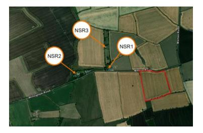
The normal criteria for indoor sound levels in residential developments (BS8233) is 35dB during the day and 30dB at night, with short duration levels not exceeding 45dB at night in bedrooms. The report includes survey results from existing (baseline) noise levels, the readings were taken during the day and night.
